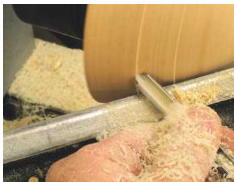
▲ Pic.3 The perfect cut with the bevel in contact with the wood. You can see that as I have gone round the bowl, I have decreased the depth of my cut and will return to the other part shortly
